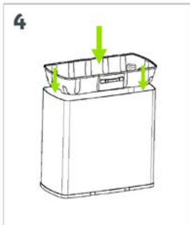
4 Place the bottom lid, rounded portion facing down into the top of the roll. This will tighten the roll from the structure and maintain stability.
