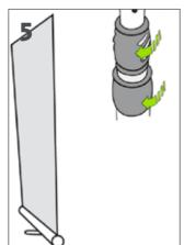
twist to the left to loosen and right to tighten the grip plastic locks.
