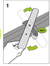
Turn the stabilizing foot perpendicular to the base until you hear it click into place.
