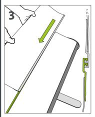
Slide the base of the graphic onto the "ECI" plastic extrusion leader strip.
