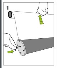
Pull the graphic and block it with the Allen Key.
