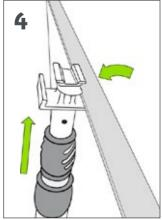
Attach the hanger onto the head Set the pole to desired height: of the pole. The pole does have light capability.
