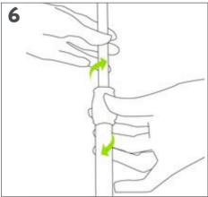
Twist to the eft to loosen and right to tighten the grip plastic locks, while adjusting the banner height.
