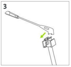
Position your optional light by sliding it into the groove of the pole head.
