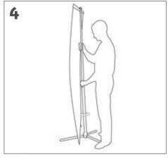
Unscrew one of the two black rings to release and adjust the telescopic pole
