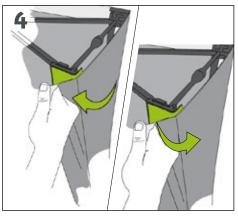
Attach the graphic to the velcro on the back of the frame. Before dismantling the structure, you must detach the graphic from the back of the structure. Warning: do not trap the graphic into the clips of the structure.
