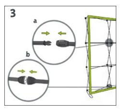
Connect the clips to lock the structure in place. Warning: unclip all connectors before taking down the display.
