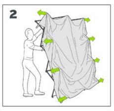
Deploy the structure while bending it slightly backwards.
