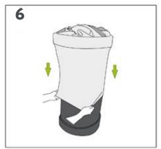
Put the graphic wrap on form the top and slide it down to cover the case.
