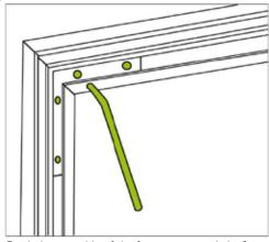
Finish the assembly of the frame on one side by fixing the 2 barkets.
