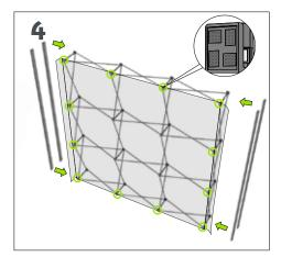
Install the bars vertically on the sides of the front and back hubs, then install the rear graphic by aligning the velcro tabs to the front of the hubs.
