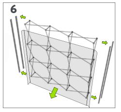
To dismantle, remove the graphics and the bars. Return the graphics to their plastic bags for storage. Separate the magnetic connectors then fold up the structure.
