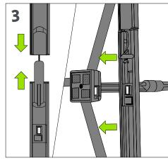
Assemble the magnetic bars and align them with the magnetics in the hubs.
