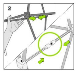
Pull the structure together at the cross-bars. The magnetic connectors will lock the frame into place.
