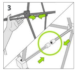
Pull the structure together at the cross-bars. The magnetic connectors will lock the frame into place.
