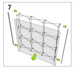
To dismantle, remove the graphic and the bars. Return the graphic to its plastic bag for storage. Separate the magnetic connectors then fold up the structure.
