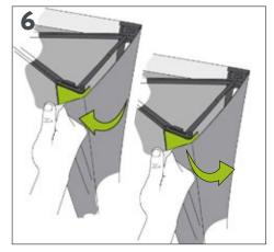
Attach the graphic's endcaps to the back of the frame.
